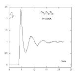
Ab-initio simulation of the radial distribution function of copper in the CuTiZr alloy
